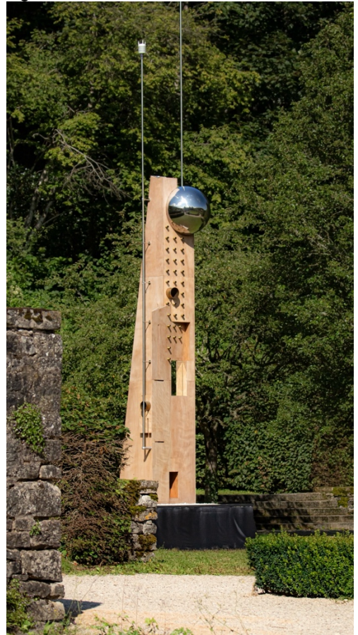
Fig. 1 – The Ithaca Dream, a meteoroelectronic instrument from our lab that transposes real time several atmospheric events (wind speed and direction, clouds height and density, temperature, pressure, humidity, pluviosity, electrostatic field, lightnings within a
